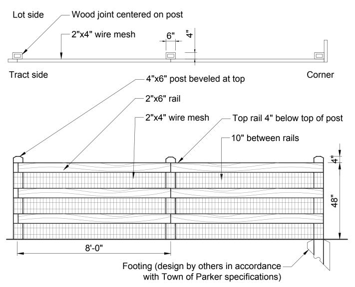
Stain Color: Semi-transparent Cape Cod Gray Wire Mesh: Galvanized 14 gauge installed between post and rail.
