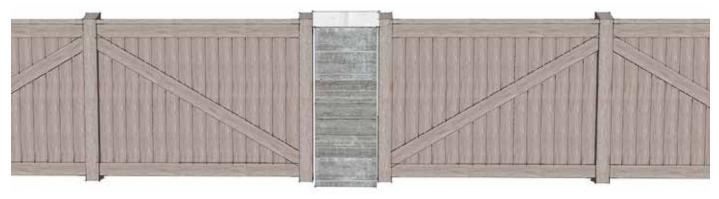
Column Height:6'-4"Cap:2'-4" squareCap Thickness:6.5"Material:Developer approved veneer
